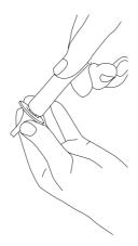
Put the boot on the floor, apply pressure using your knee to hold it in place. Push the pin all the way in using the grease tube nozzle.
