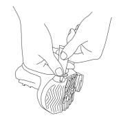
Stop applying pressure to the grease tube before removing it from the boot. Repeat this process 2-3 times on each side of the boot to fully lubricate the pins.
