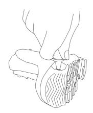
Squeeze the grease tube hard for 10 seconds, and make sure the nozzle seals against the mechanism so that grease does not leak.
