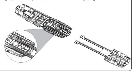
Mounting the binding: Lift the Quicklock. Slide the rear of the binding house onto the front of the mounting plate. The tracks on the underside of the binding house should grasp the tracks on the sides of the mounting plate. The heel needs to grasp the heel of the mountingplates. Slide the binding until "0", neutral position, appears in the window. Close the Quicklock and you are ready!
