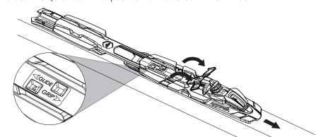
For better glide: Lift the Quicklock and push the binding backwards to preferred position, choose between three different positions, -1. -2, -3 for better glide. Close the Quicklock. The position is indicated in the window.
