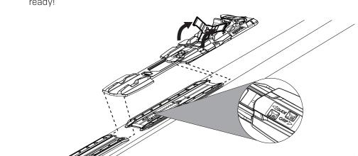
For better grip: Lift the Quicklock and push the binding forwards to preferred position, choose between three different positions, +1, +2, +3 for better grip. Close the Quicklock. The position is indicated in the window.
