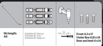
Match correct shoe size, mount the jigg with black BC-insert onto the ski, matching the balance point (1). Drill using the advised drill bit (2), remove the jigg and use binding glue into the holes (3).
