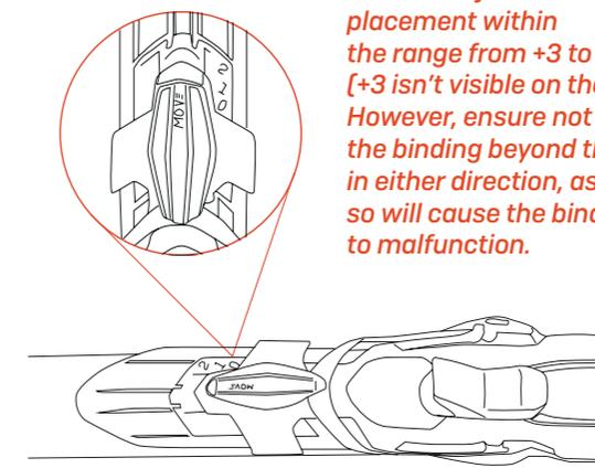
The MOVE handle serves two main purposes: it locks the opening and closing mechanism, and it allows for adjustment of the binding position.
