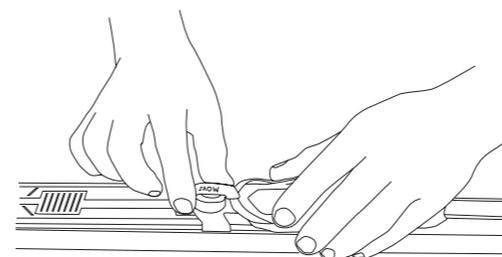
Push the binding forward until it stops. Turn the handle counter clockwise as shown in the illustration below, as you continue pushing the binding forward.
