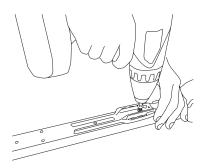
Place the binding house on the binding heel aligning the binding house holes with the drilled ones in the roller ski. Use the screws included and screwt he house into place. Tighten by hand.
