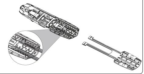
**For better grip:** Lift the Quicklock and push the binding forwards to preferred position, choose between three different positions, +1, +2, +3 for better grip. Close the Quicklock. The position is indicated in the window.
