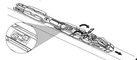
**4. For better glide:** Lift the Quicklock and push the binding backwards to preferred position, choose between three different positions, -1. -2, -3 for better glide. Close the Quicklock. The position is indicated in the window.
