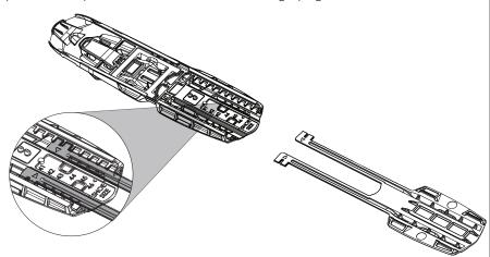
**2. Mounting the binding:** Lift the Quicklock. Slide the rear of the binding house onto the front of the mounting plate. The tracks on the underside of the binding house should grasp the tracks on the sides of the mounting plate. The heel needs to grasp the heel of the mountingplates. Slide the binding until "0", neutral position, appears in the window. Close the Quicklock and you are ready!
