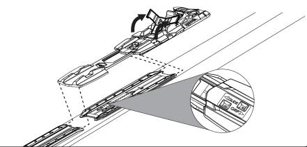
**3. For better grip:** Lift the Quicklock and push the binding forwards to preferred position, choose between three different positions, +1, +2, +3 for better grip. Close the Quicklock. The position is indicated in the window.
